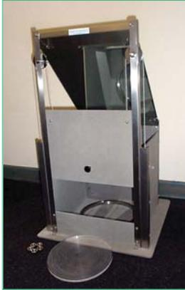
The WIRA Flammability Tester is used to test the effects of a small source of ignition on floorcoverings. It can be used for either the hot metal nut test (BS 4790) or the methenamine tablet test (ISO 6925 and BS 6307).
