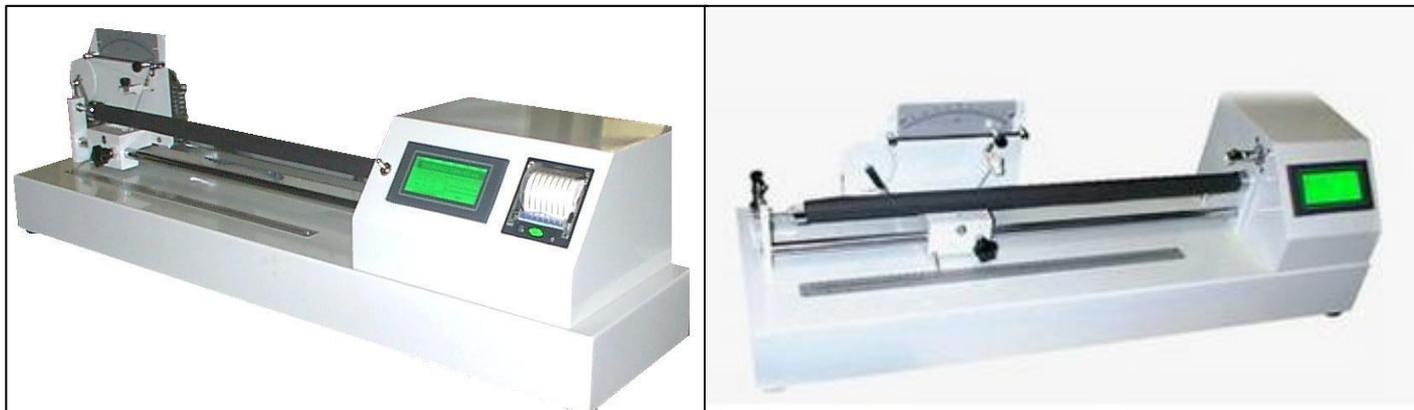
This instrument is used to determine twisting values of single and twisted yarns in compliance with standard **UNI EN ISO 2060 - ISO 2061 - ASTM D1423 - ASTM D1422**.
