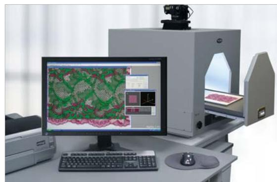
Using controlled, consistent and defined illumination conditions, DigiEye captures and measures product colour and appearance with an amazingly high resolution and great precision.
