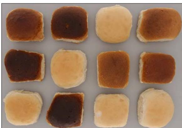
The image of bread rolls above illustrates diverse variations in the crust colour of a selection of bread rolls. These rolls can be images with DigiEye individually or as a group to produce appearance standards for crust colour.
