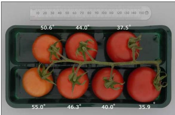
One of the significant advantages of the DigiEye system is, due to the consistency of the images taken, direct comparisons can be made between images taken of product in different locations worldwide and at different times.
