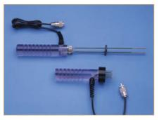
Traditional type hand-held moisture testers use simple probes that can be susceptible to the effects of inconsistent sample density, particularly where textile fibres are concerned.
