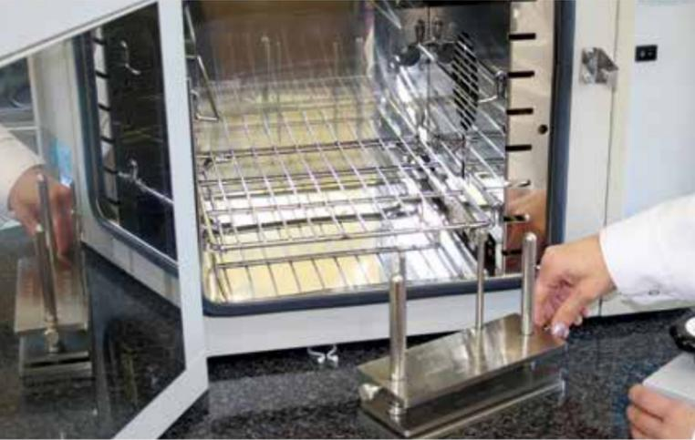
**The Perspirometer applies a specified pressure to a series of test specimens separated by acrylic or glass plates.**
